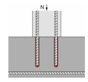
b) Overlap joint at a foundation of a column or wall
