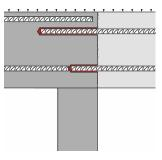
(a) Overlap joint for rebar connections of slabs and beams
