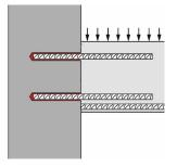
(c) End anchoring of slabs or beams (simply supported)
